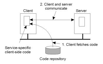
The principle of dynamically configuring a client to communicate to a server. The client first fetches the necessary software, and then invokes the server.
