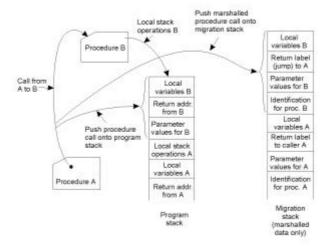
The principle of maintaining a migration stack to support migration of an execution segment in a heterogeneous environment
